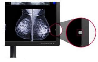
Built in front sensors eliminate the need for bulky photometers and manual, time-consuming calibration and conformance testing. All DBI displays are bundled with the CFS<sup>™</sup> Calibration software suite for automatic DICOM calibration, conformance testing, report generation, MQSA testing, reporting and non-conformance alerts via the web.
