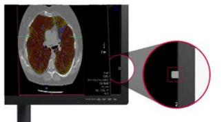
Built in front sensors eliminate the need for bulky photometers and manual, time-consuming calibration and conformance testing. All DBI systems/solutions are bundled with the CFS<sup>™</sup> Calibration software suite for automatic DICOM calibration, conformance testing, report generation, reporting and non-conformance alerts via the web.
